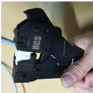
Make sure the jack is firmly placed. Terminate wires with punch down tool
