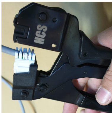
Make sure the jack is firmly placed. Terminate wires with punch down tool
